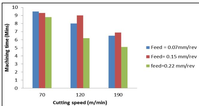
**Fig 6:** Machining time for tool under dry conditions
