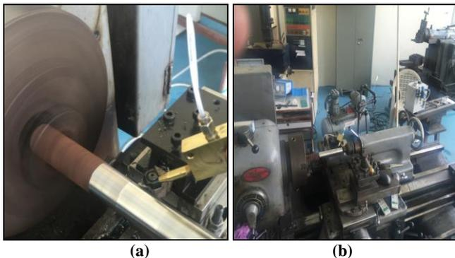
Fig 1: (a) Nozzle used in MQL setup, (b) MQL setup used with lathe machine
