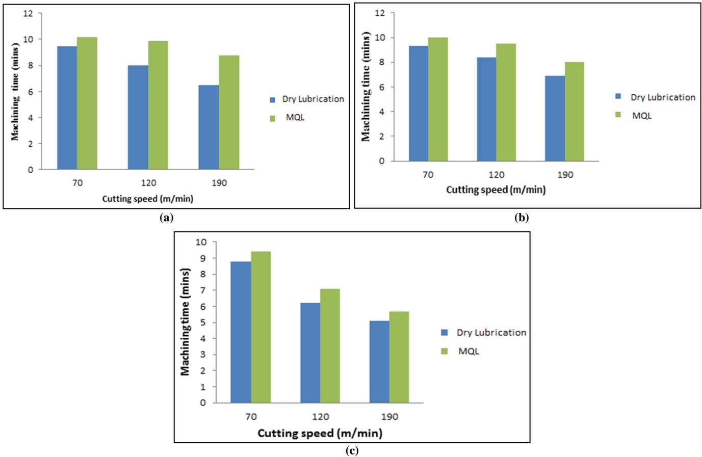
Fig 9: Machining time when feed rate is (a) 0.07 mm/rev (b) 0.15 mm/rev and (c) 0.22 mm/rev
