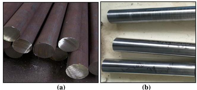
Fig 2: AISI 4340 Steel rod (a) Unfinished (b) Finished
