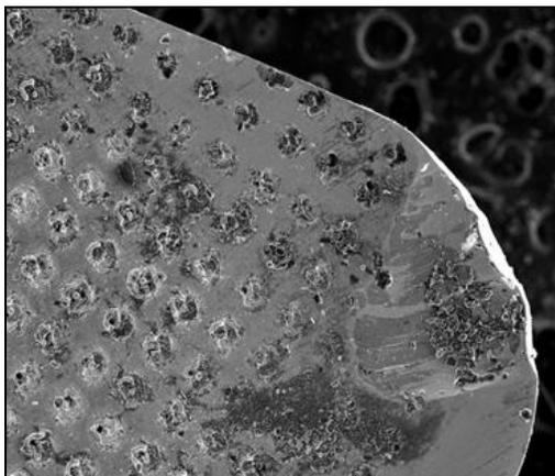
**Fig 4:** Failure of tool at 55 HRC
