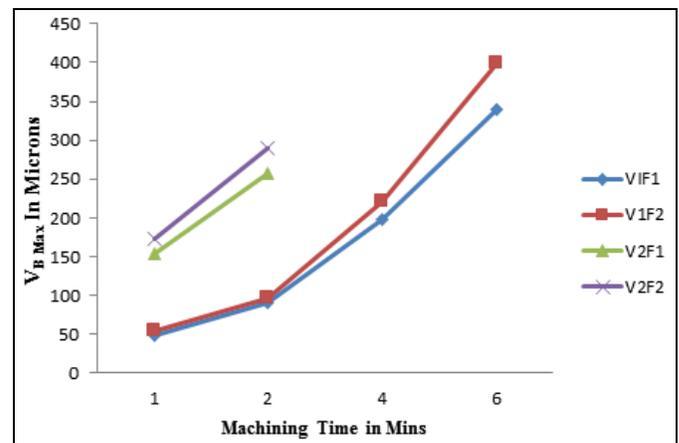
**Fig 5:** Flank wear
