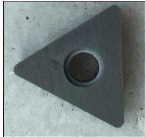
**Fig 3:** Tool Insert TNMA 160408-THMF (WIDIA)
