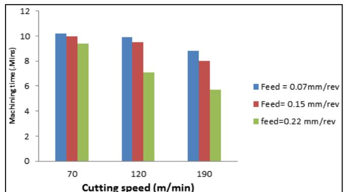
**Fig 7:** Machining time for tool using minimum quantity lubrication.
