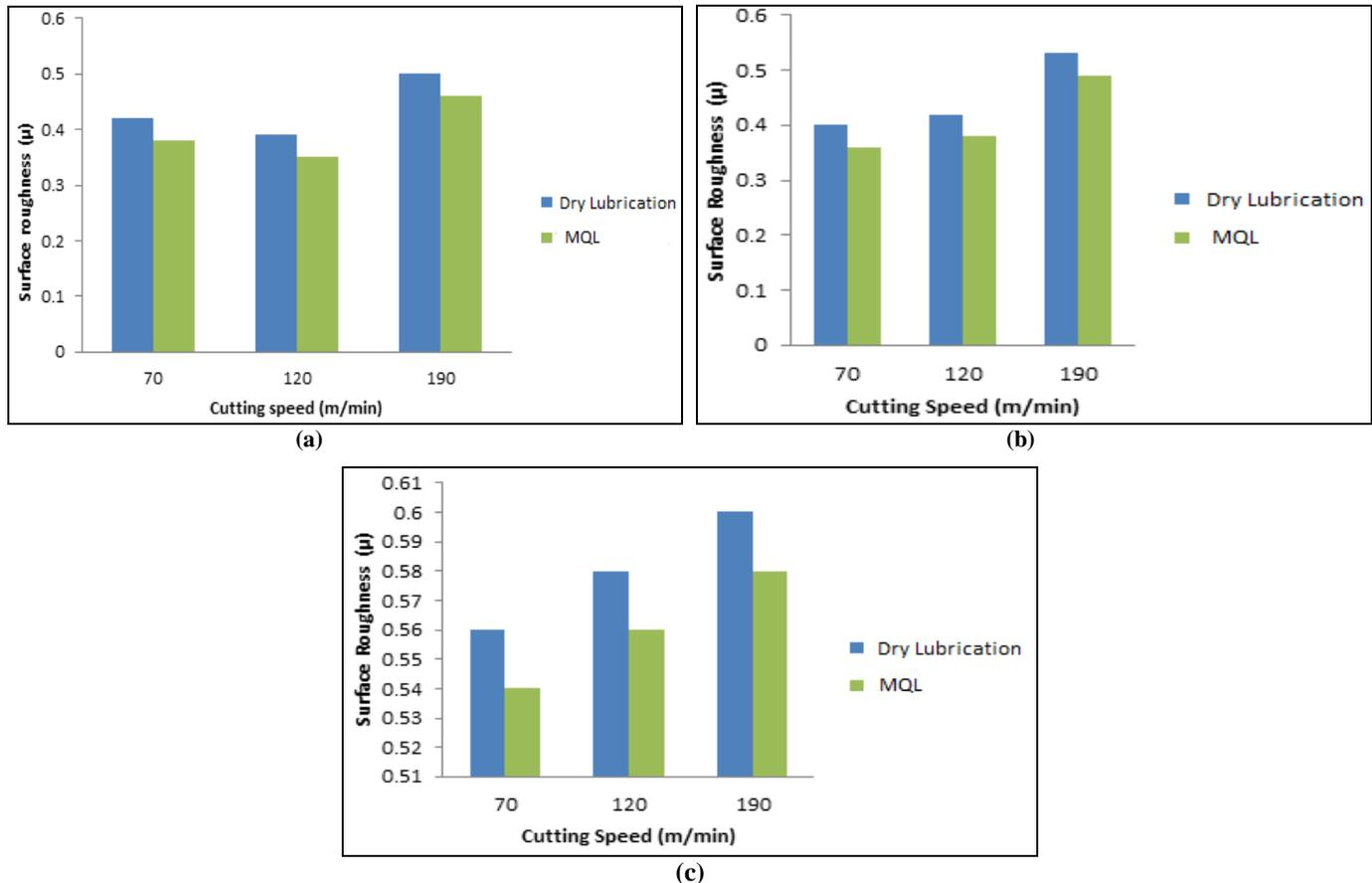
Fig 10: Surface Roughness feed is (a) 0.07 mm/rev (b) 0.15 mm/rev and (c) 0.22 mm/rev
