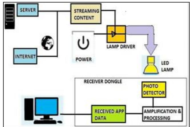
Fig 4: Data transmission using LED [6].
