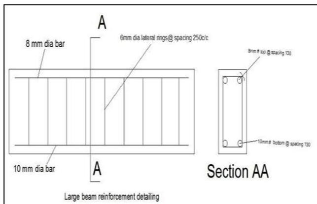
**Fig 4:** Large Beam detailing
