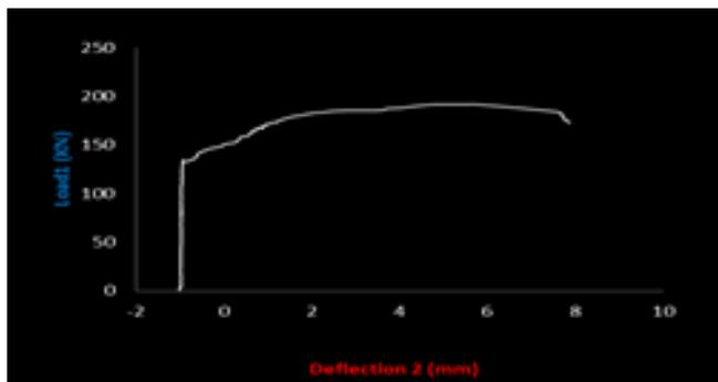
Fig 10: Deflection curve of conventional beam
