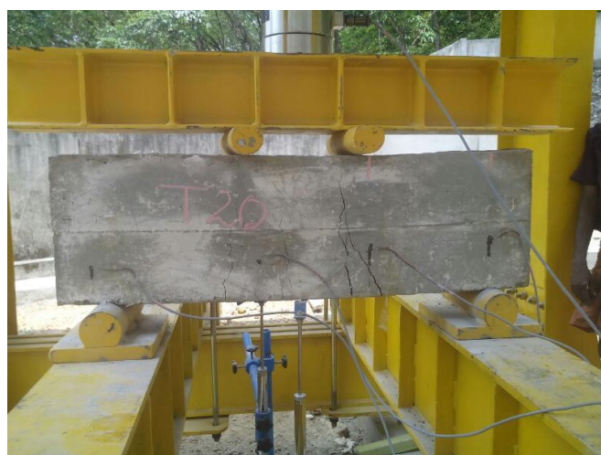
Fig 6: Testing of beam specimens
