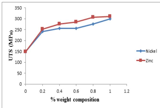
**Fig 6:** Effect of alloy compositions on the UTS of tin bronze (Cu-10%Sn)
