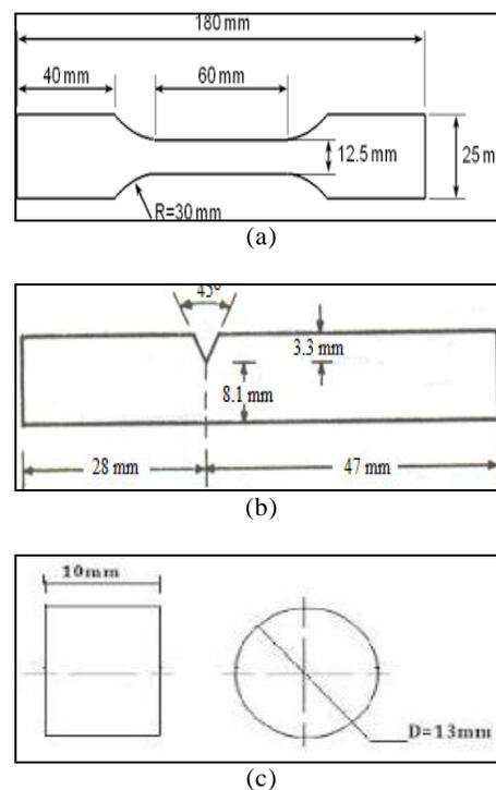
**Fig 2:** (a) Tensile test specimen (b) Notch impact test specimen, (c) Hardness/microstructure specimen.
