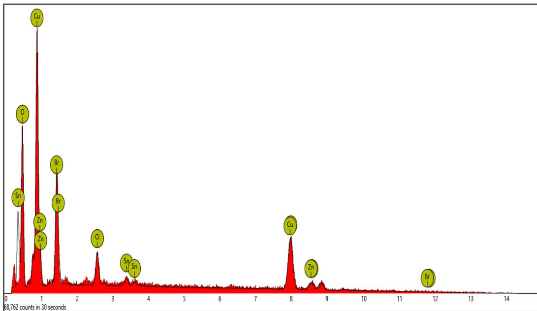
Fig 5: EDS spectrum of Cu-10%Sn-1%Zn alloy
