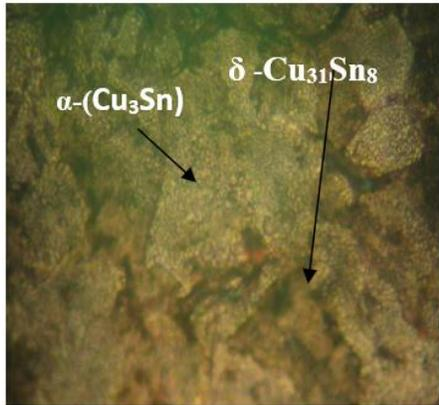
**Plate 1:** Cu-10%Sn alloy (Control)
