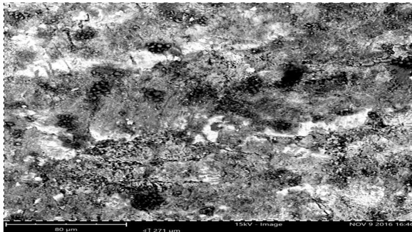
**Plate 14:** SEM micrograph of Cu-10%Sn + 1%Zn alloy
