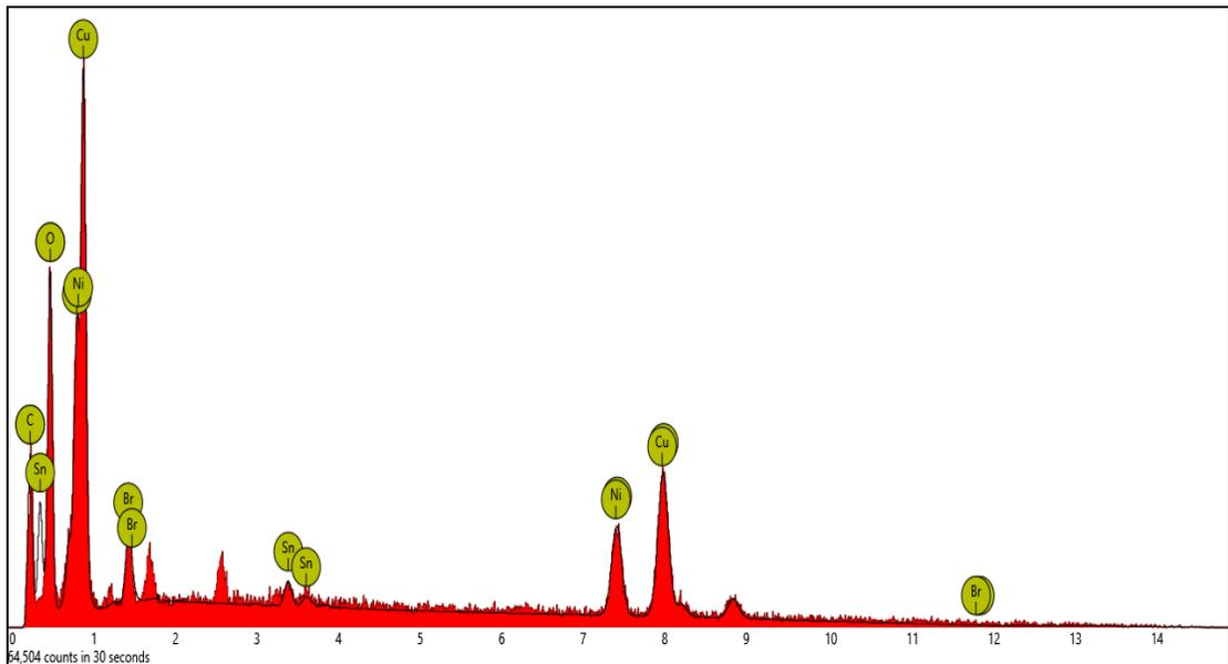
Fig 4: EDS spectrum of Cu-10%Sn-1%Ni alloy
