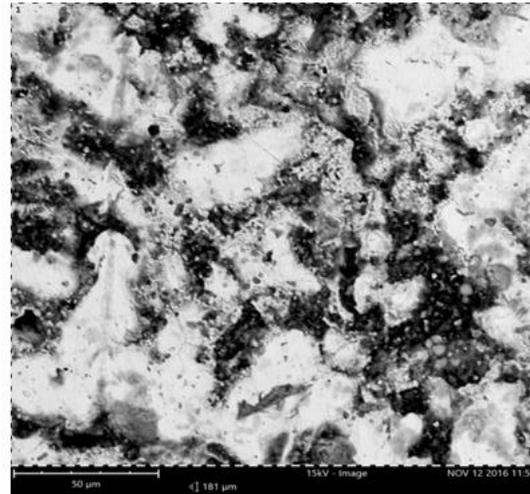
**Plate 13:** SEM micrograph of Cu-10%Sn + 1%Ni
