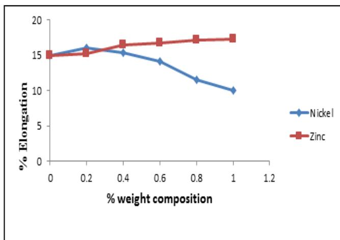
**Fig 7:** Effect of alloy compositions on the % elongation of tin bronze (Cu-10%Sn)
