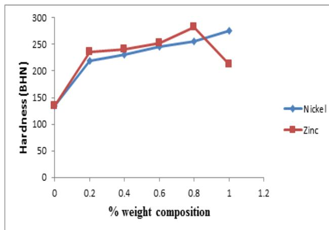
**Fig 8:** Effect of alloy compositions on the hardness of tin bronze (Cu-10%Sn)
