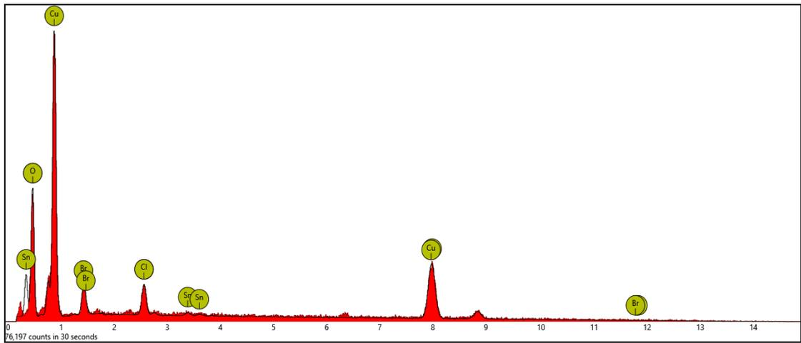
Fig 3: EDS spectrum of Cu-10%Sn alloy
