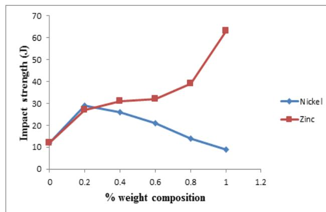
**Fig 9:** Effect of alloy compositions on the impact strength of tin bronze (Cu-10%Sn)
