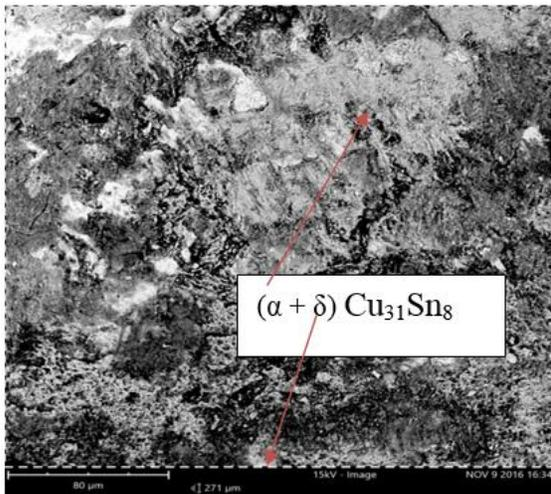
**Plate 12:** SEM micrograph of Cu-10%Sn alloy (Control)
