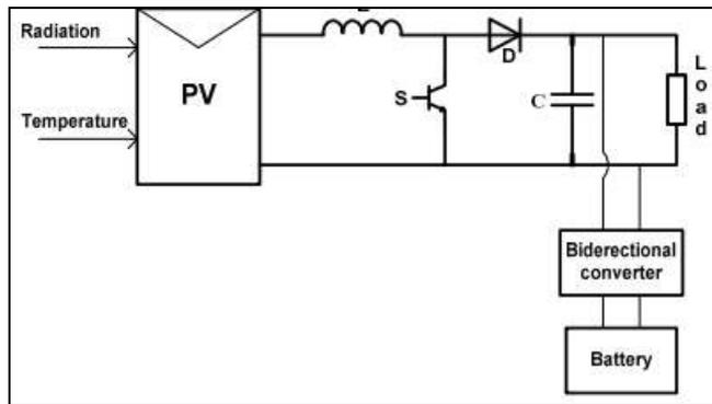
Fig 3: Typical configuration of stand-alone PV system
