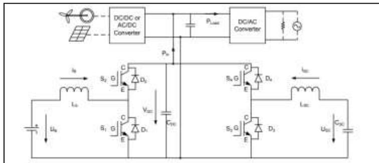
**Fig 1:** Proposed Super-Capacitor Hybrid System
