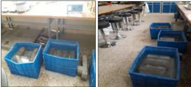
Fig 4: Curing pots in the laboratory
