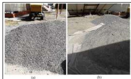
**Fig 3:** crushed gravel (a coarse and b fine) used for the concrete mix
