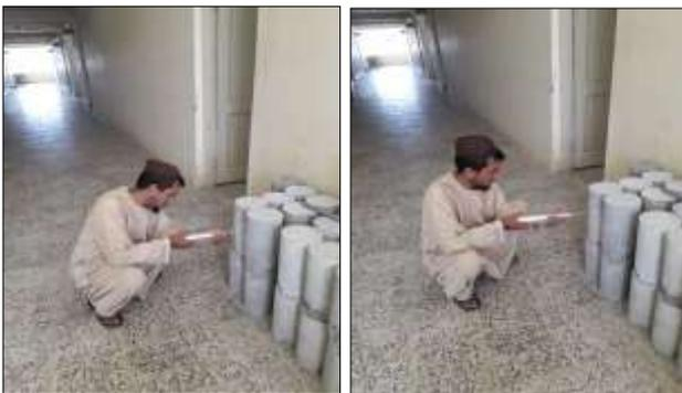
Fig 5: Cylindrical specimen test conditions by the Schmidt hammer
