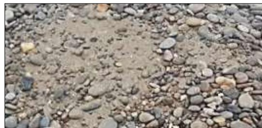
**Fig 2:** Helmand River gravel used for the concrete mix
