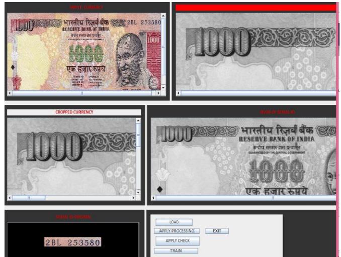
Fig 4: Serial number extraction the above fig. shows that how Indian currency gets processed and its Serial number is located on note, Cropped for display purpose. Blurred images are also displayed in two of the windows.
