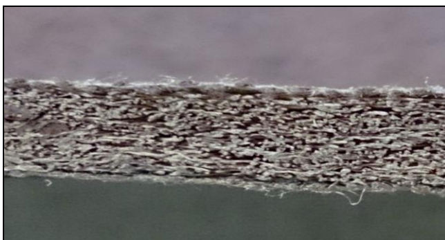
Fig 3: Nonwoven Banana sample with double side polyester fabric, polyurethane and polypropylene layering
