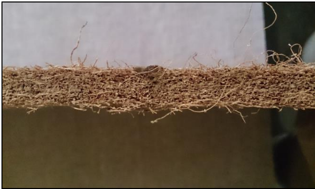
Fig 1: Nonwoven Banana sample without polyester fabric, polyurethane and polypropylene layering
