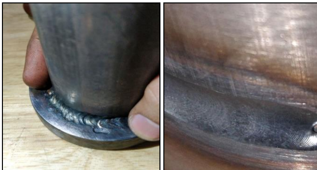
Fig 1: Manual Weld Joint
