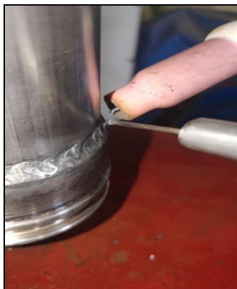
Fig 9: Weld Joint Obtained
