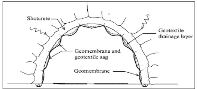
**Fig 12:** Tunnel Waterproofing
