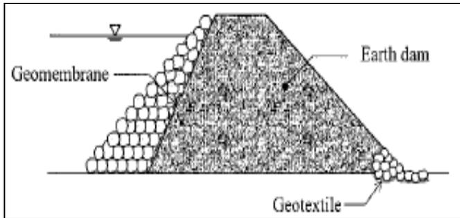
**Fig 11(A):** Geomembrane Waterproofing of Earth or Earth-Rock Dam Face
