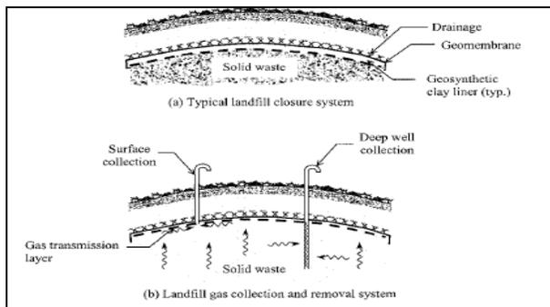
**Fig 15:** Geosynthetic for Landfill Closure Systems
