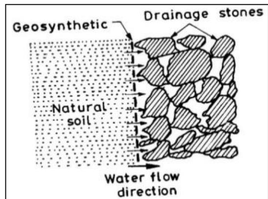
Fig 4: Basic Mechanism Involved In the Filtration Function
