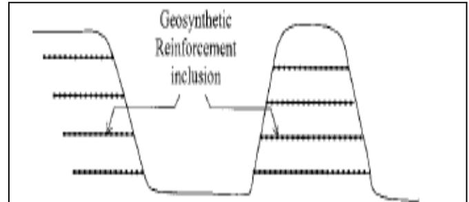
**Fig 7:** Soil Slope Reinforcement
