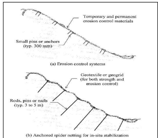
**Fig 13:** Geosynthetic for Erosion Control
