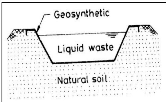
**Fig 6:** Basic Mechanisms Involved in the Fluid Barrier Function
