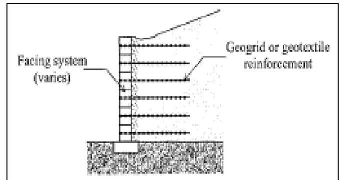
**Fig 8:** Geosynthetic Reinforced Wall
