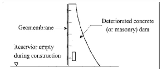
**Fig 10:** Geomembrane waterproofing of dams
