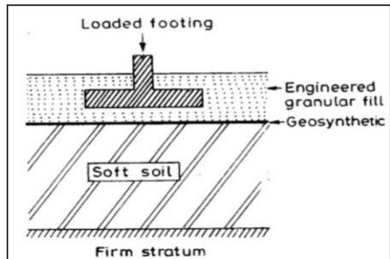
Fig 3: A Loaded Geosynthetic-Reinforced Granular Fill-Soft Soil System
