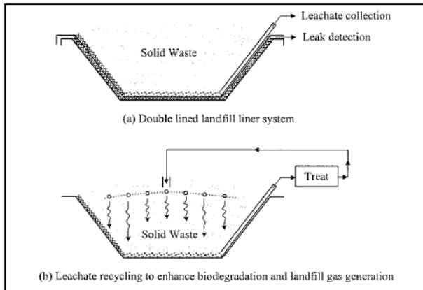
**Fig 14:** Geosynthetic for Landfill Liner System
