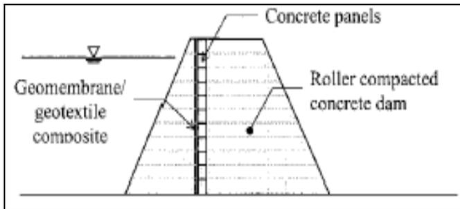
**Fig 11(B):** Geomembrane Waterproofing Of Roller Compacted Concrete Dam
