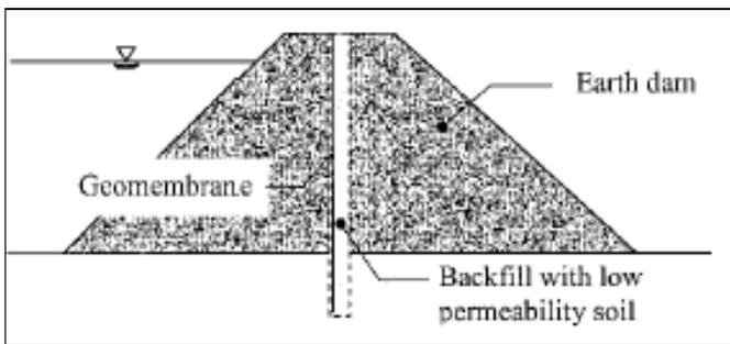
**Fig 11(C):** Geomembrane Waterproofing Of Existing Dam
