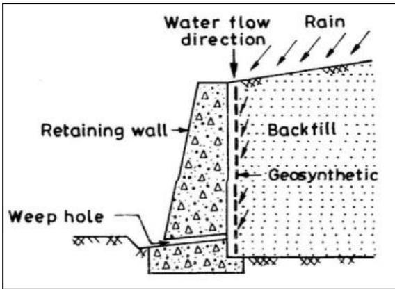
**Fig 5:** Basic Mechanisms Involved In the Drainage Function
