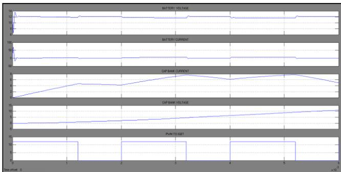
Fig 9: Buck Operation Waveforms
