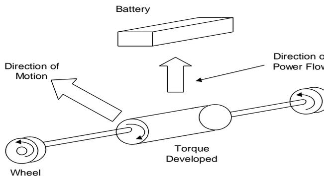
**Fig 2:** Regenerative action during braking
