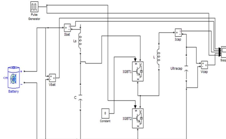
Fig 8: Braking Circuit Model
