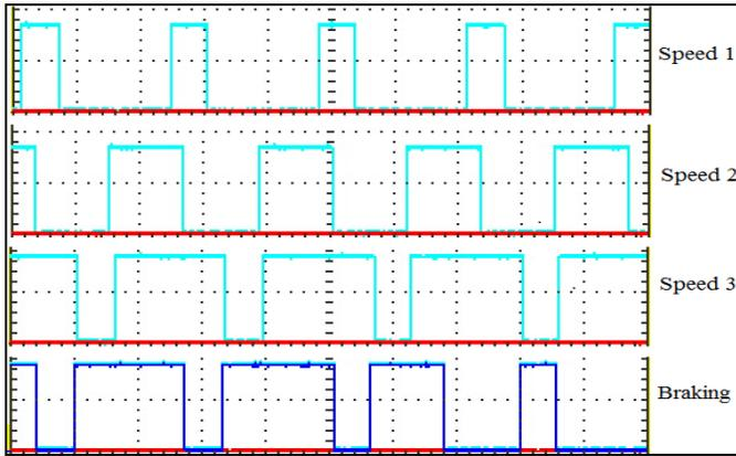
Fig 7: Buck Operation Waveforms
