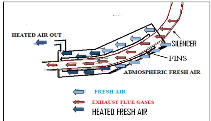
Fig 1: Schematic diagram of air preheater
