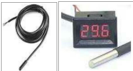
Fig 7 Actual Image Thermocouple Scanners and Wire
