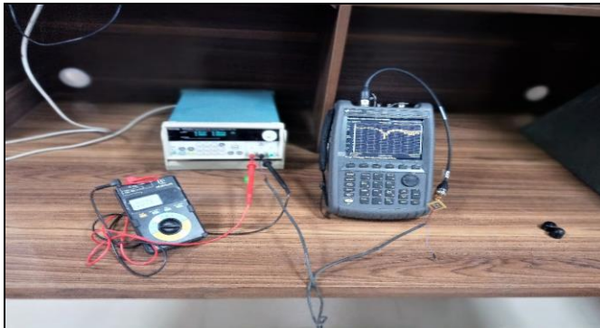
Fig 7: Antenna return loss measurement w. r. to voltage setup
